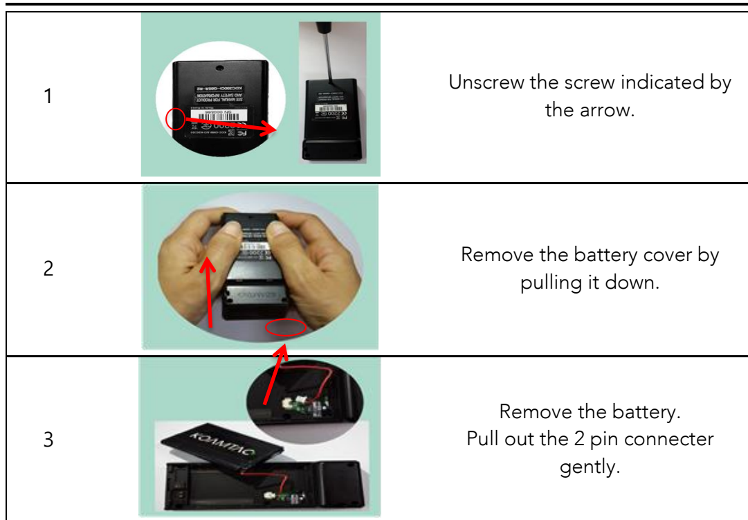
Figure 15 - Replacing a Battery
