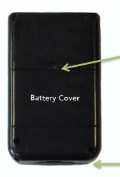
Remove the battery cover screw on the back of the KDC200/KDC250.KDC300. A longer screw will be included in your order.
