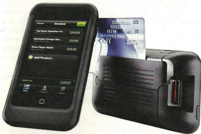
The Linea Pro gives an iPod touch both a barcode scanner and magnetic stripe reader.
